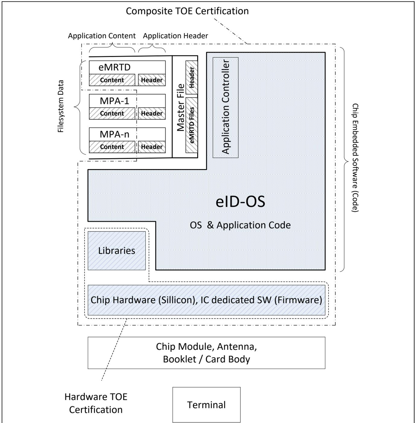
Figure 1 TOE block diagram
