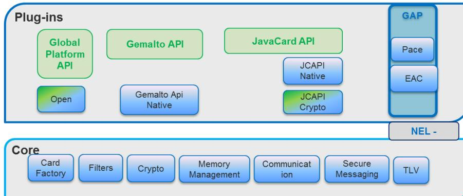
**Figure 3: MultiApp V4.1 Java Card platform architecture**
