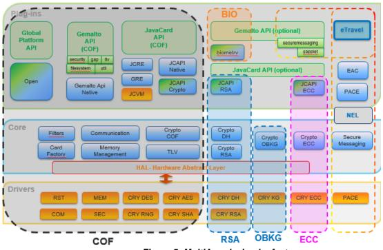
Figure 5: MultiApp design by features
