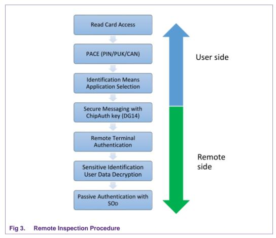
S.PACE-Terminal performs the Remote Inspection Procedure (see Fig 3) and therefore (i) contains a terminal for the communication with the eDigitalIdentity document's chip, (ii) implements the terminal part of the PACE protocol, (iii) authenticates the eDigitalIdentity holder to the eDigitalIdentity document using a shared password (PIN, PUK or CAN), and (iv) implements the Chip Authentication Protocols Version 1 according [13].
