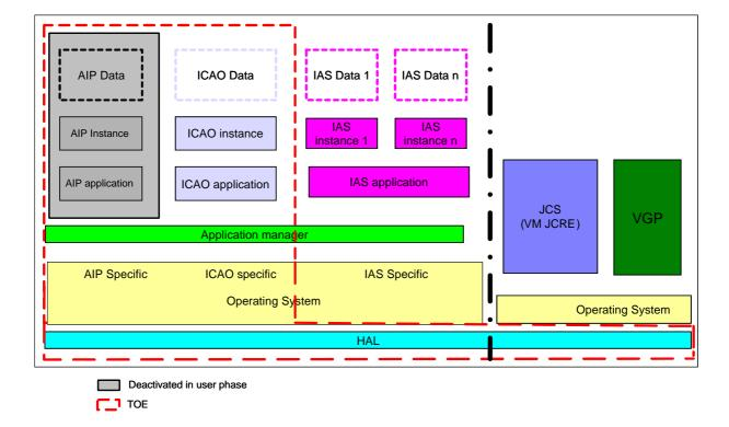
The evaluation facility verified the isolation between the various applications, notably between those in the TOE with those not included in the TOE. The evaluation facility verified that a Java applet could only access to its own data and not to those belonging to another applet.
