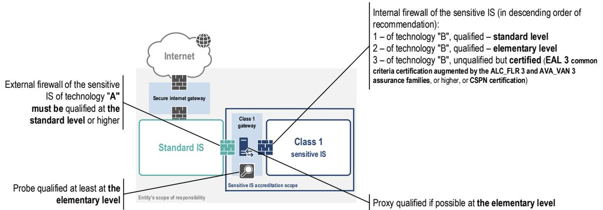
Figure 10 – Sensitive IS of class 1 - Example of a physically partitioned IS architecture : positioning of security devices
