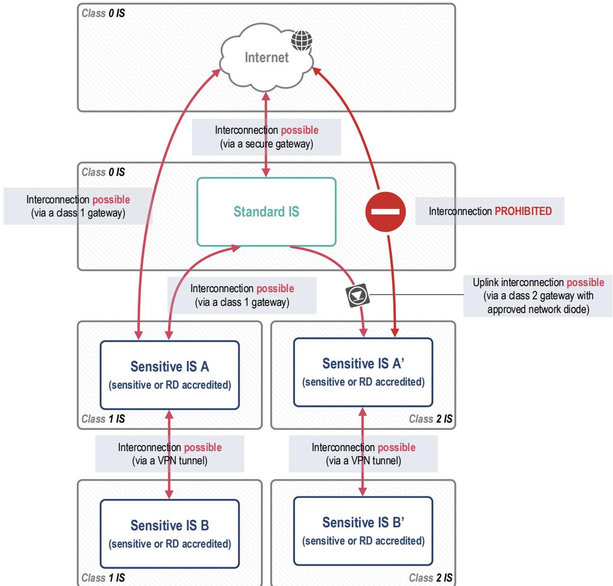
Figure 2 – Mapping of IS classes (0, 1 or 2) to the levels of sensitivity of the ISs (public, standard, sensitive, RD)
