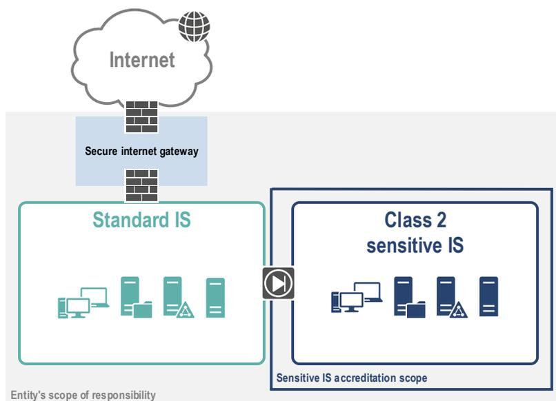
Figure 5 – Sensitive IS of class 2 - Example of an architecture with a direct one-way interconnection via an uplink gateway
