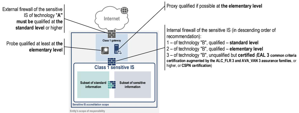
Figure 11 – Sensitive IS of class 1 - Example of an architecture with logical partitioning of sensitive and standard information : positioning of security devices
