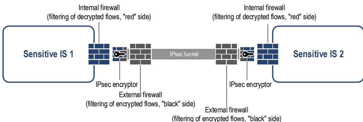
Figure 9 – Architecture of an interconnection between sensitive ISs
