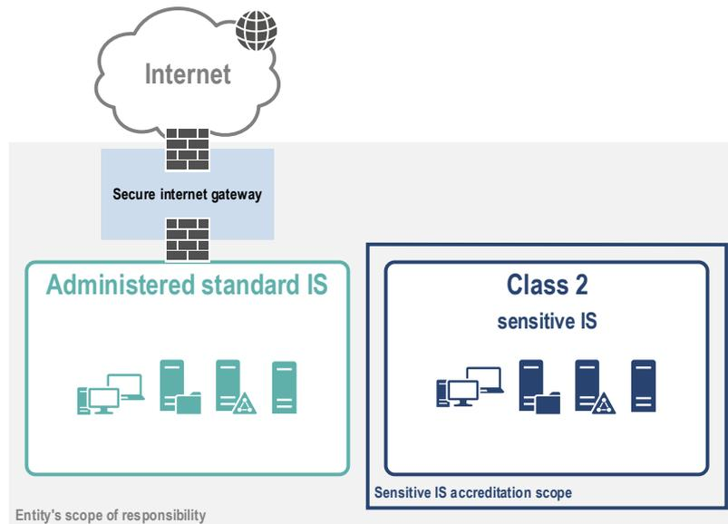
Figure 6 – Sensitive IS of class 2 - Example of an architecture without direct interconnection
