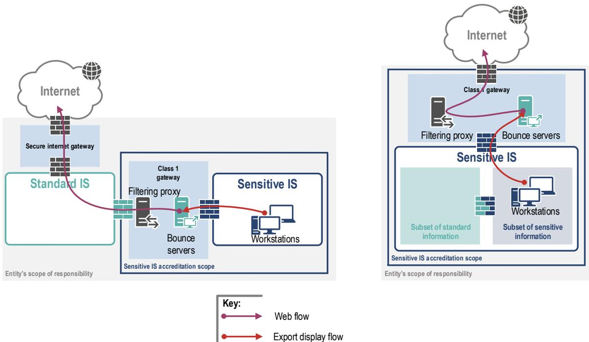
Figure 12 – Web browsing : examples of architectures for an IS of class 1, with bounce servers (left: case of a physically partitioned architecture; right: case of an architecture with logical partitioning of sensitive and standard information)
