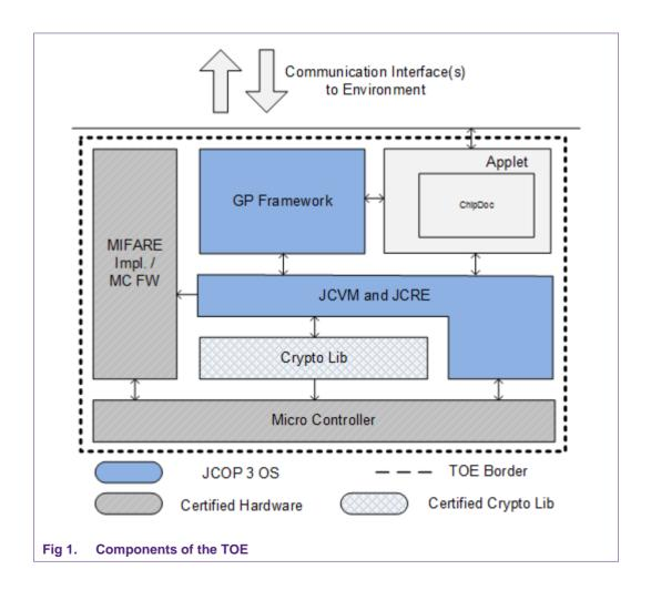
The TOE consists of an applet which is executed by a software stack that is stored on a Micro Controller. For a complete picture of the TOE see Fig 1, and for details with regards to the different components see section 1.3.1.
