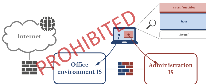
Figure 4.4: Office environment station hosting a virtual administration machine
