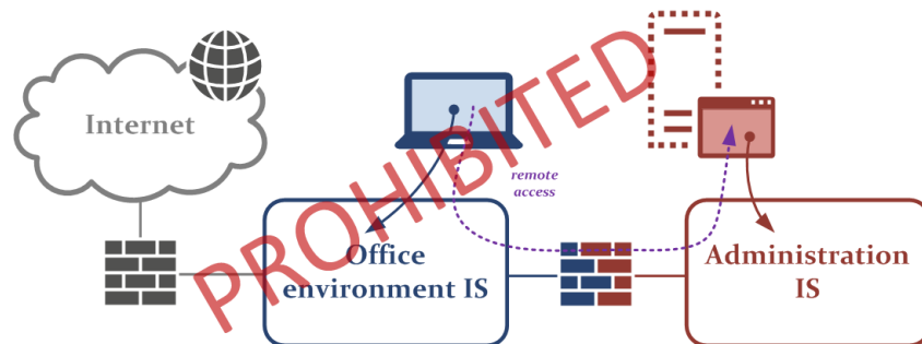
Figure 4.6: Physical office environment station with remote access to a virtualised administration environment
