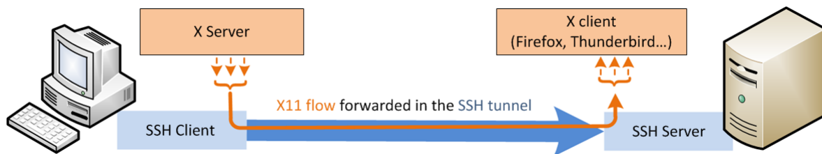
Figure 3: Diagram of X11 forwarding through SSH
