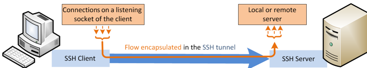
Figure 1: Diagram of a flow forwarding on the SSH client
