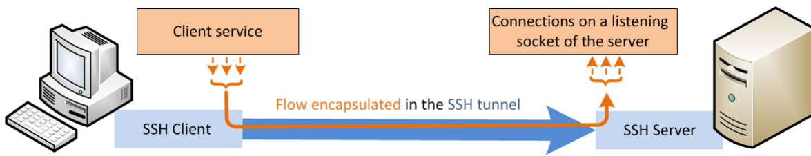
Figure 2: Diagram of a flow forwarding on the SSH server
