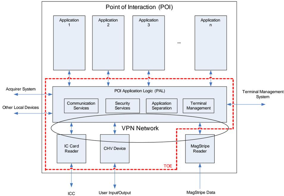
**Figure 1 Configuration POI-CHIP-ONLY**
